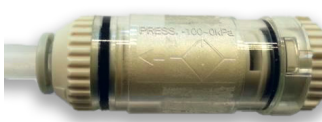
Put the core back in place and close the filter. Note the direction of air flow (towards the sensor). Open the regulator on the gas cylinder and let the gas flow for approximately one minute without the calibration adapter connected to the sensor, then close the regulator.
