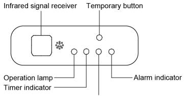
PRE-DEF indicator(cooling and heating type) or fan only indicator(cooling only type)
