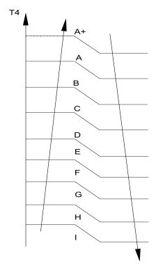
While A,B,C...means different fan speed of outdoor unit.
