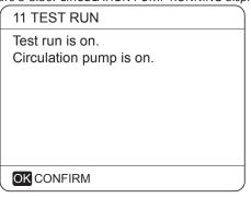
will operate. After a further 2 min the flow switch start to check the water flow. If the water flow rate is sufficient, both PUMPI and PUMPO operate until the next command is received. If the water flow rate is insufficient over any 15-second period, PUMPI and PUMPO stop and error code E8 is displayed. Refer to Part 3, 8.2 "Error Code table".
