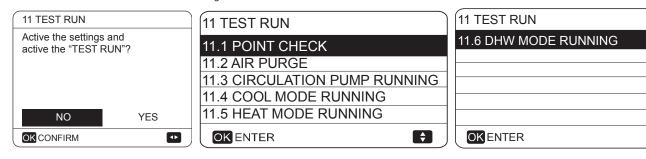
During test run, all buttons except OK are invalid. If you want to turn off the test run, please press OK. For example ,when the unit is in air purge mode, after you press OK, the following page will be displayed:
