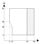
Figure 2-6.3: Domestic hot water operating limits<sup>1</sup>
