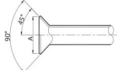
When connecting a flared joint, apply some compressor oil to the inner and outer surfaces of the flared opening to facilitate the connection and rotation of the flare nut, ensure firm connection between the sealing surface and the bearing surface, and avoid the pipe becoming deformed.
