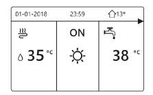
**ROOM TEMP.** sets whether space heating/cooling modes are controlled according to the room temperature detected by the temperature sensor in the Matrix Split user interface. If **YES** is selected, the user is able to set the room temperature set temperature on the user interface's main screen, no matter what is the setting of **WATER FLOW TEMP.**
