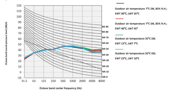
Figure 2-8.5: ATS14T octave band levels
