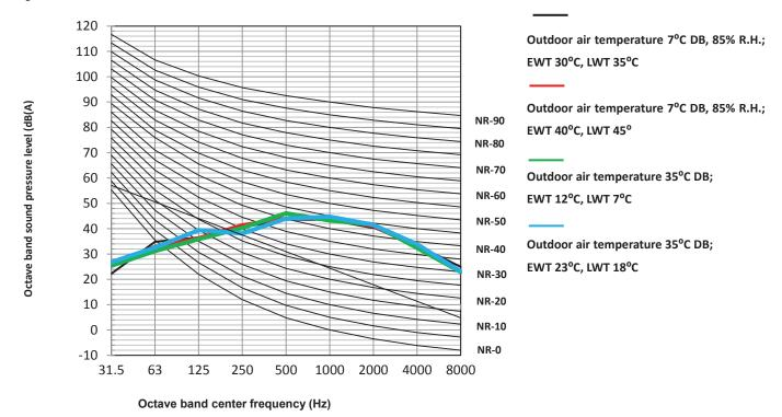
Figure 2-8.5: ATS10S octave band levels
