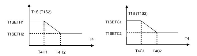
The setting of T1SETH1, T1SETH2, T4H1, T4H2 refer to Part 3, 8.6" HEATING MODE SETTING Menu" and T1SETC1, T1SETC2, T4C1, T4C2 refer to Part 3, 8.5" COOLING MODE SETTING Menu".
