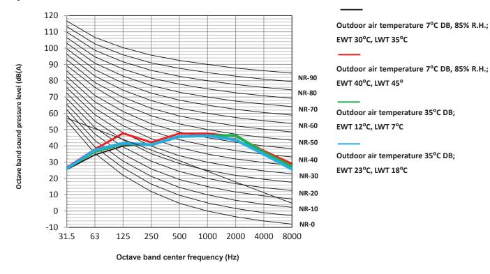
Figure 2-8.5: ATS14S octave band levels
