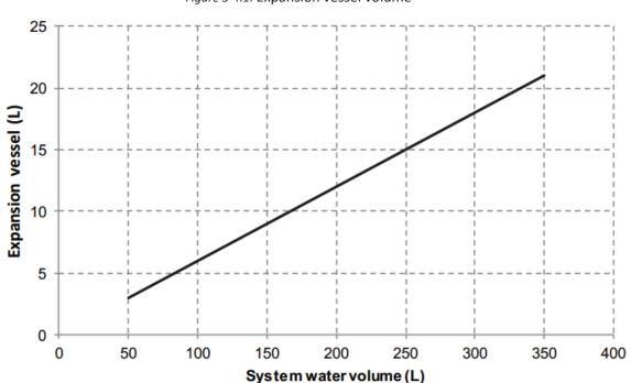
Figure 3-4.1: Expansion vessel volume
