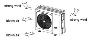
If turn the air outlet side toward the building's wall, fence or screen. Make sure there is enough room to do the installation
