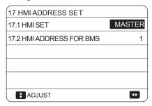
HMI SET sets the wired controller is master or slave. (0=MASTER, 1=SLAVE)
