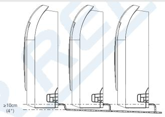
In order to ensure smooth drainage, the height difference between the wall outlet and the hanging plate must be greater than 470mm.
