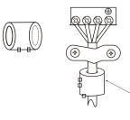
Pass the belt through the hole of the Magnetic ring to fix it on the cable
