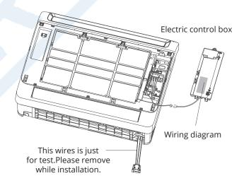
**NOTE:** When taking out the electric control box, pay attention to loosen and remove the terminal.
