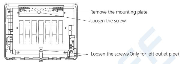
NOTE: If the pipe comes out on the left, it is necessary to loosen the screws on the bottom mounting plate. If the pipe comes out in other directions, it is not necessary.
