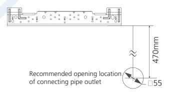
Drainage pipe fixing requirements When installing the drainage pipe (not provided ), please fix it with a tie or rope.
