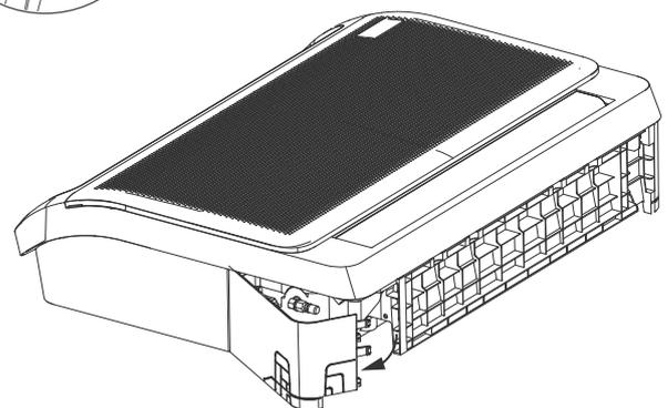
NOTE: In order to drain smoothly, the position of the drain pipe must refer to the above figure when discharging the right pipe.
