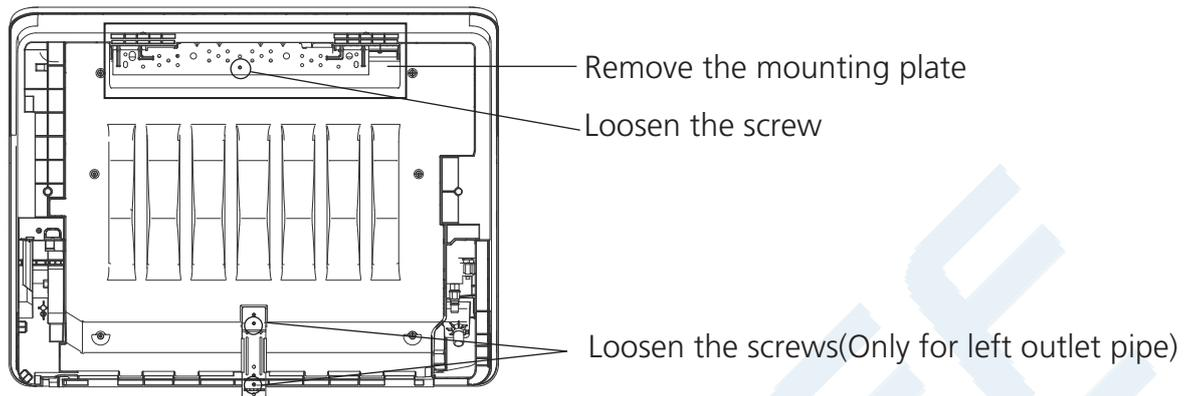
NOTE: If the pipe comes out on the left, it is necessary to loosen the screws on the bottom mounting plate. If the pipe comes out in other directions, it is not necessary.
