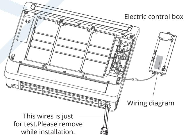
**NOTE:** When taking out the electric control box, pay attention to loosen and remove the terminal.
