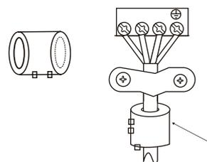
Pass the belt through the hole of the Magnetic ring to fix it on the cable
